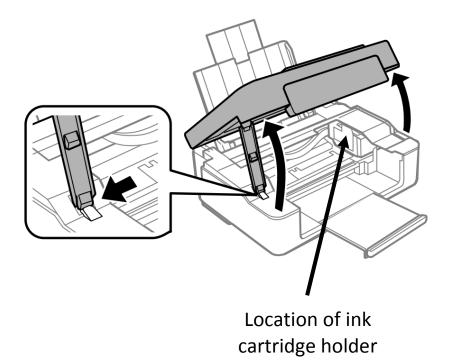
The top half of the printer latches open. Push the blue catch on the left hand side to allow the top half of the printer to close again.
