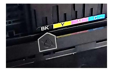
Press the Stop Printing button again. The cartridge holder will either move a little, so the bump aligns with another empty cartridge, or the holder will move to the right, ready to have the cartridge or cartridges replaced.
