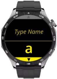
The Synapptic on-screen keyboard is specially designed for simplicity and ease of use on a small screen, where a full-sized keyboard wouldn't be practical. Instead of displaying all the keys at once, it shows just one character at a time.
